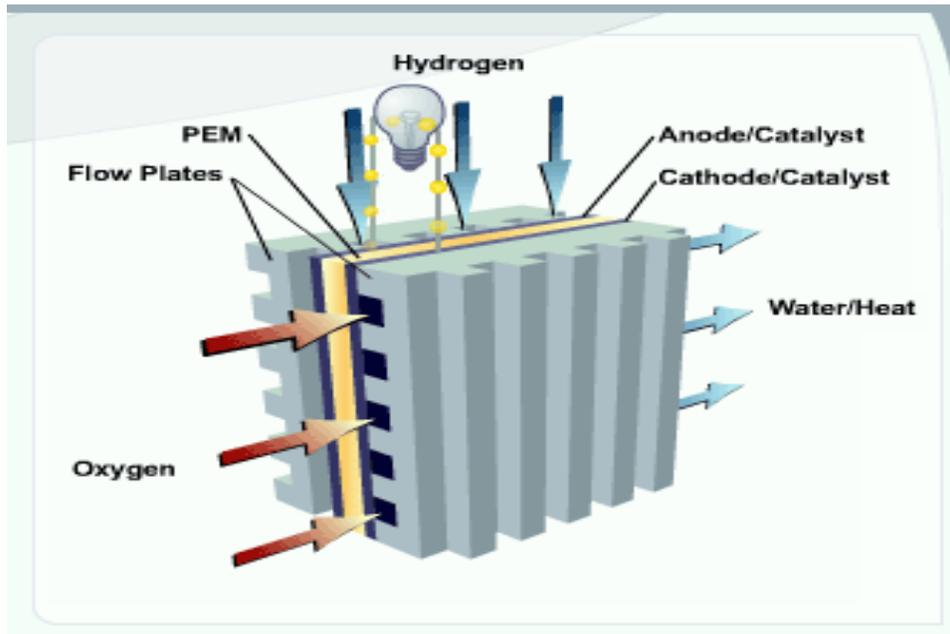
PEM fuel cells work with a polymer electrolyte in the form of a thin, permeable sheet. Efficiency is about 40 to 50 percent, and operating temperature is about 80 degrees C. Cell outputs generally range from 50 to 250 kW. The solid, flexible electrolyte will not leak or crack, and these cells operate at a low enough temperature to make them suitable for homes and cars. But their fuels must be purified, and a platinum catalyst is used on both sides of the membrane, raising costs.
