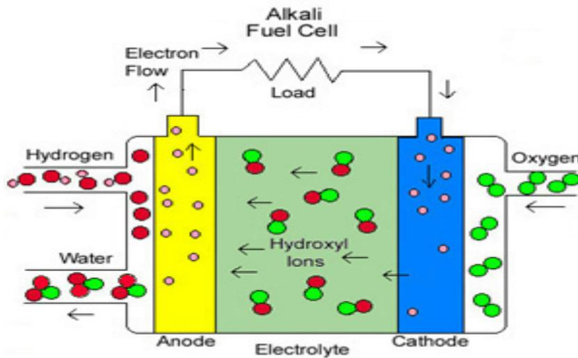
Alkaline fuel cells (AFC) are one of the most developed technologies and have been used since the mid-1960s by NASA in the Apollo and Space Shuttle programs. The fuel cells on board these spacecraft provide electrical power for on-board systems, as well as drinking water. AFCs are among the most efficient in generating electricity at nearly 70%.
