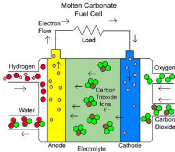
Molten-carbonate fuel cells (MCFCs) are high-temperature fuel cells, which operate at temperatures of 600°C and above. They have the highest efficiencies of any type fuel cell, including solid oxide fuel cells, proton exchange membrane fuel cells and phosphoric acid fuel cell and are not subject to the high-temperature material issues that affect solid-oxide technology.
