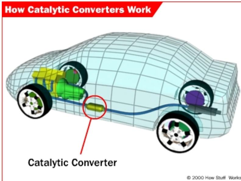
**Illustration 1: The location of catalytic converters in a car**
